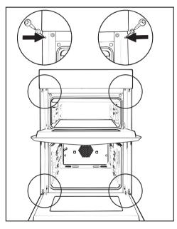
■ Open the oven door and using four screws secure the oven to the side walls of the housing unit through the holes in the oven trim.
